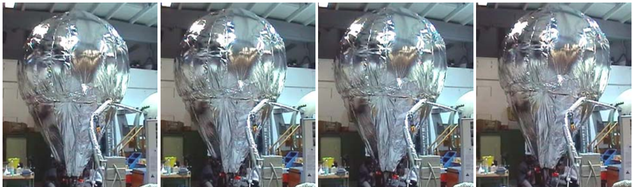
Fig. 12: Sequence during the first take off. After lifting the ballast weights, the balloon took off, and moved smoothly towards the ceiling.
